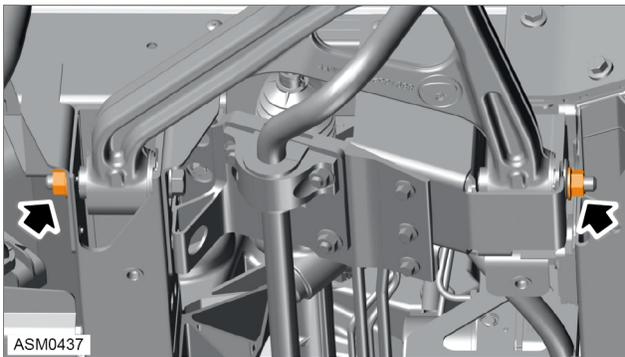
3. Loosen M12 nuts (x2) securing lower wishbone to front subframe.
