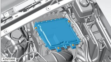
2. Remove 6x20 screws (x4) securing ECM to airbox assembly. **Torque 6 Nm.**
