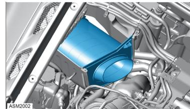
9. Remove air filter element.
