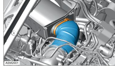
7. Release hose clamp securing air inlet hose to air filter element. **Torque 3 Nm.**
