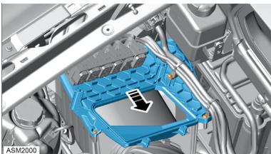
5. Remove 5x20 screws (x3) securing airbox lid to airbox assembly. **Torque 1.2 Nm.**
